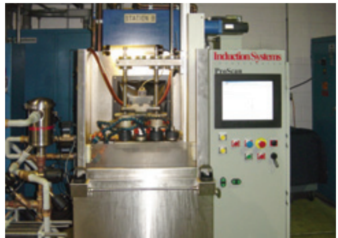
Fig. 3 Recently installed dual-spindle induction scanner
